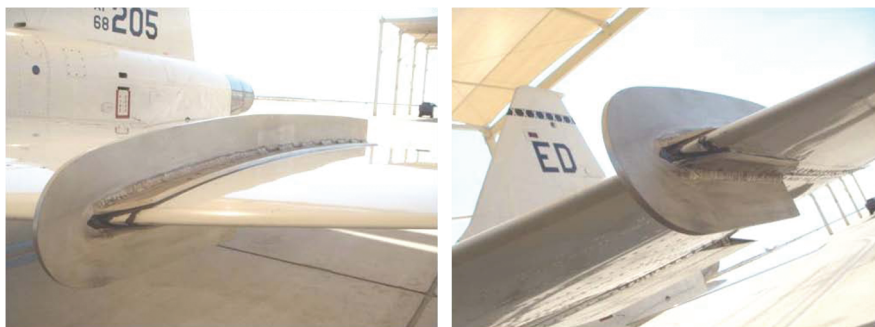
Fig. 5 Flight-test wing fence as installed on aircraft.
