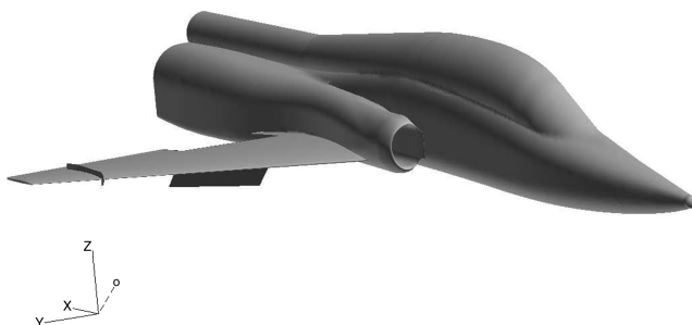
Fig. 1 CFD-modeled T-38 geometry with fence.
