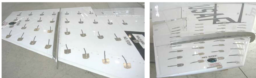
Fig. 6 Flight-test tufts, as placed on aircraft (front view and side view).
